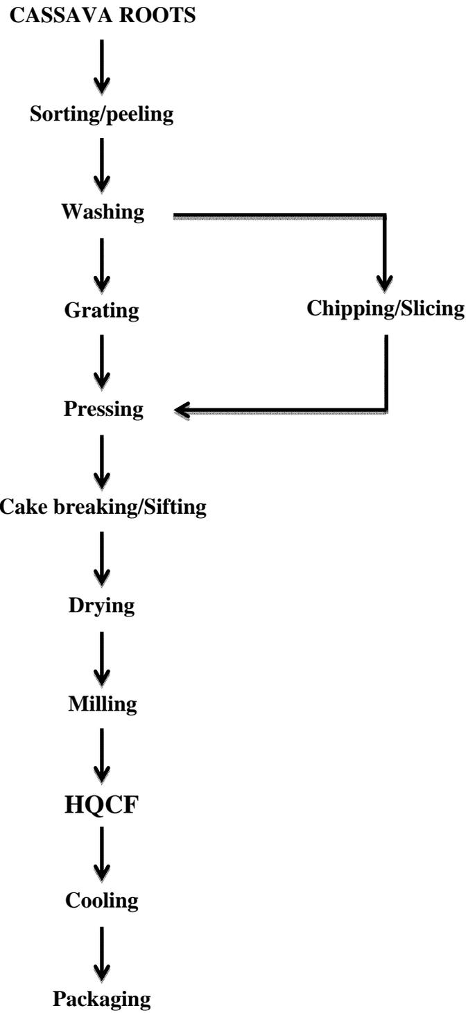
Figure 1: Flow diagram for processing cassava roots into HQCF
