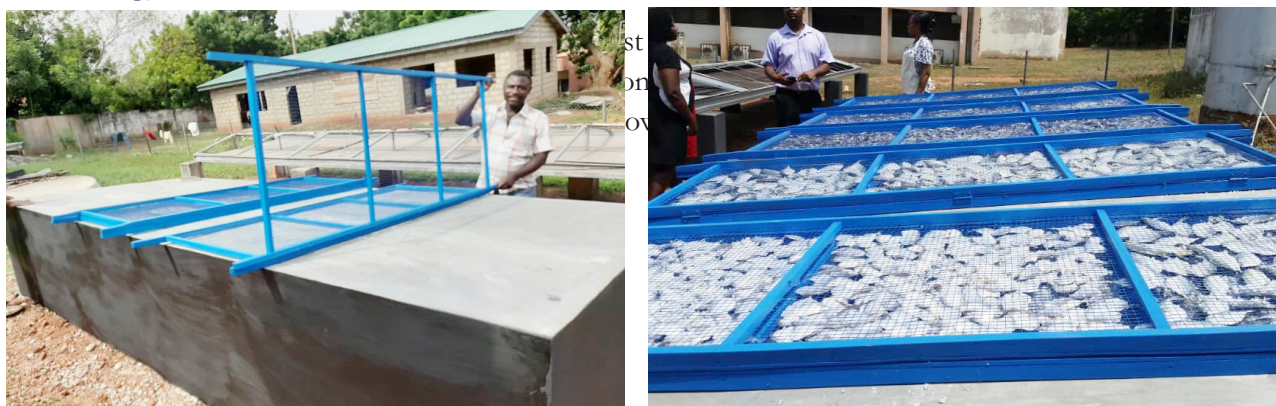
Pilot scale drying platform and racks constructed at CSIR-FRI
